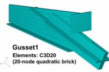
Fig. 11 Finite element mesh of Gusset 1
