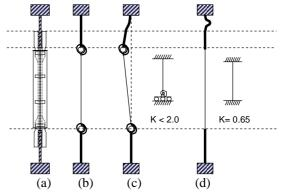
Fig. 6 Brace boundary conditions and buckling modes
