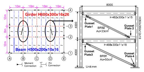
Fig. 8 Floor framing plan and BRBF elevation
