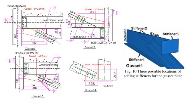
Fig. 9 Details at the gusset plate connections
